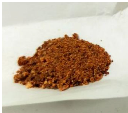
Figure 1. The synthesized ferrous fumarate obtained from the reaction between FeSO 4 and disodium fumarate
